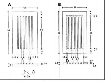
Figure 1. Top view and cross-section of the plastic slot maker (A) and plastic cover piece (B). All dimensions are in millimeters. An enlarged view of a cross-section of the tooth is shown in the lower part of panel (A). The area within the dotted lines in the diagram of the cover piece in panel (B) is 0.7mm thick whereas the border area outside the dotted lines is 1.0mm thick.
